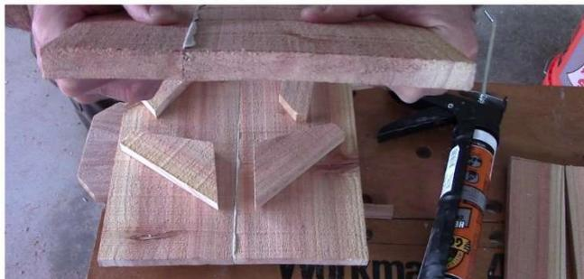
For assembling the pieces, glue the floor and roof to the side pieces. Then, set the house on a flat surface. Apply pressure to the roof (without moving it). And drive in 2 nails on each side. Repeat for the floor.
